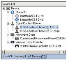
Figure 3: Detect and classify interfering sources
